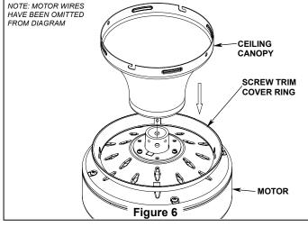
7. Alight the 3 big slots in the canopy to the 3 screws in the motor coupler. Firmly attach the canopy cover to the motor with the three screws removed in step 5 and steel washers from the part bag. (Figure 7)
