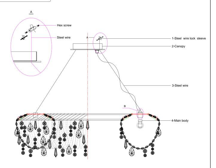
The dash area of the wire — lock sleeve is flexible, when it shrinks in ,the safety wire's length can be adjusted.
