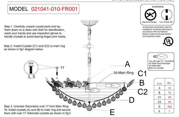
Step 4. Install 1 crystal (E) to bottom center of distributor 15
