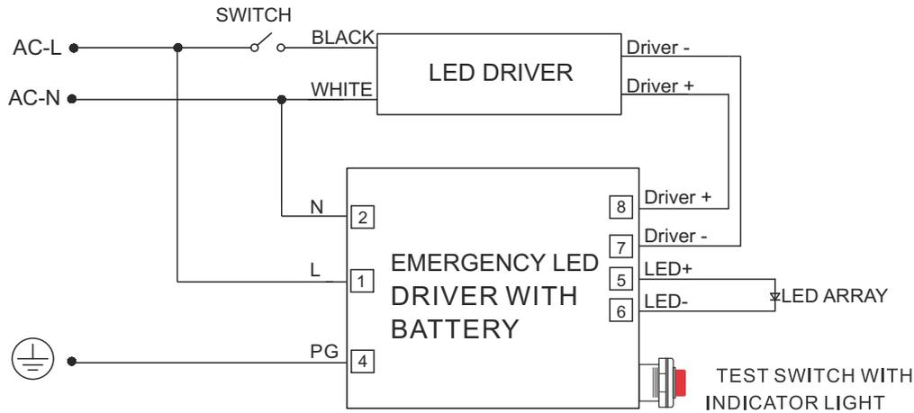
1. DO NOT MATE CONNECTOR UNTIL INSTALLATION IS COMPLETE AND AC POWER IS SUPPLIED.
